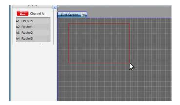
Step 4-Release the mouse. System creates a channel A4 as the size and position of the frame. You can change the size and position of the channel freely afterwards.
