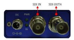
DC IN: 12V 1A. Power socket with fixing lock
